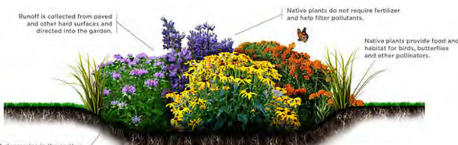
Typical Bioswale/Rain Garden
