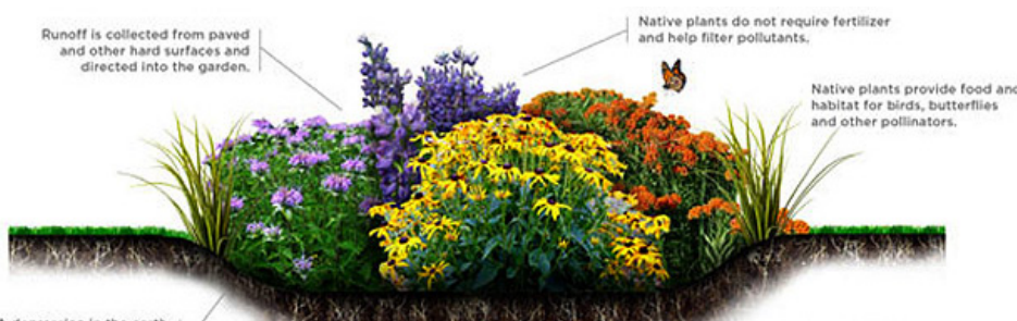
Typical Bioswale/Rain Garden
