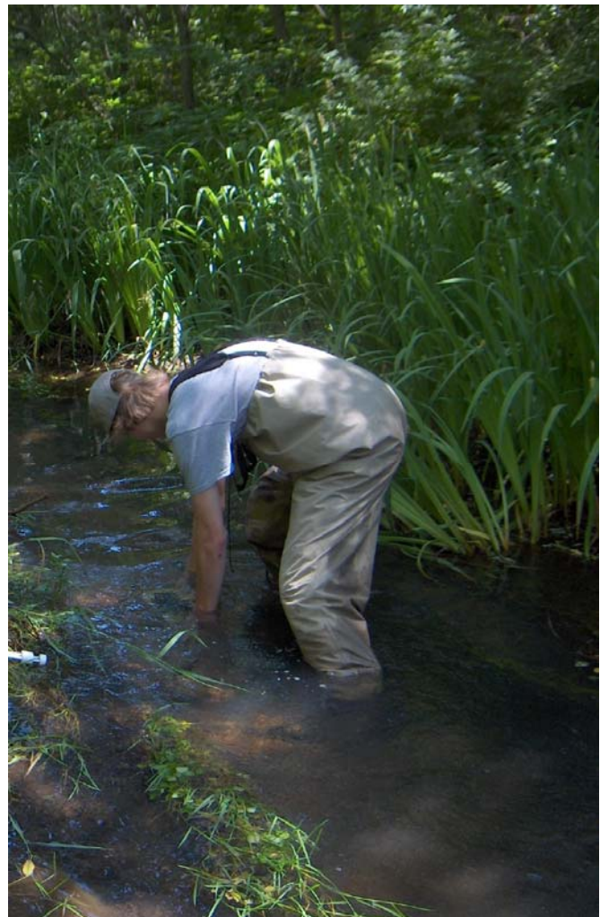
Figure 1. MBI personnel retrieving a Hester-Dendy sampler from a stream.
