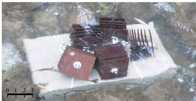
Figure 3: Hester-Dendy sampler placed into the stream bed.
