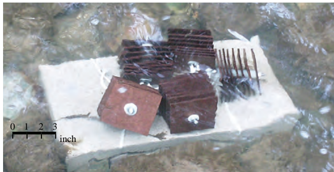
Figure 4: Hester-Dendy sampler placed into the stream bed.
