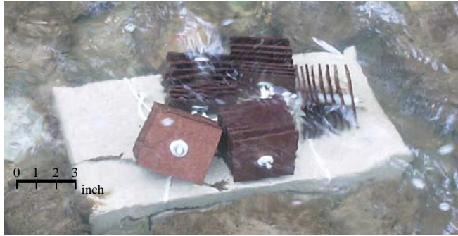
Figure 4: Hester-Dendy sampler placed into the stream bed.
