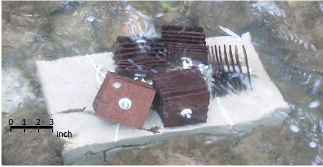
Figure 4: Hester-Dendy sampler placed into the stream bed.
