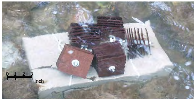
Figure 4: Hester-Dendy sampler placed into the stream bed
