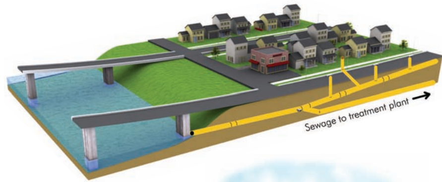
During dry weather, all sewage is carried to the treatment plant.
