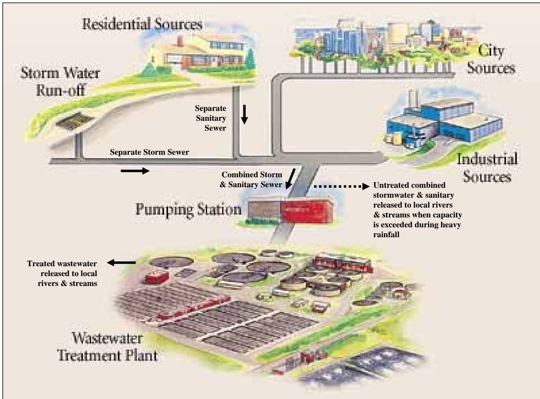
General configuration of the Elkhart Combined Sewer System
