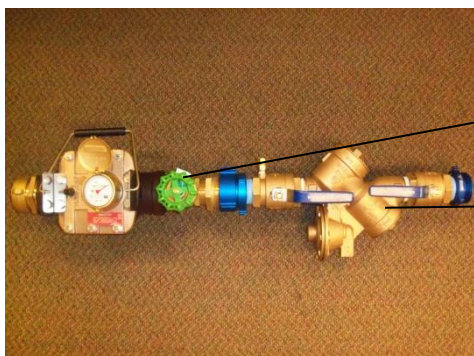
3. Hydrant meter with control valve to connects 2 1/2 " nozzle
