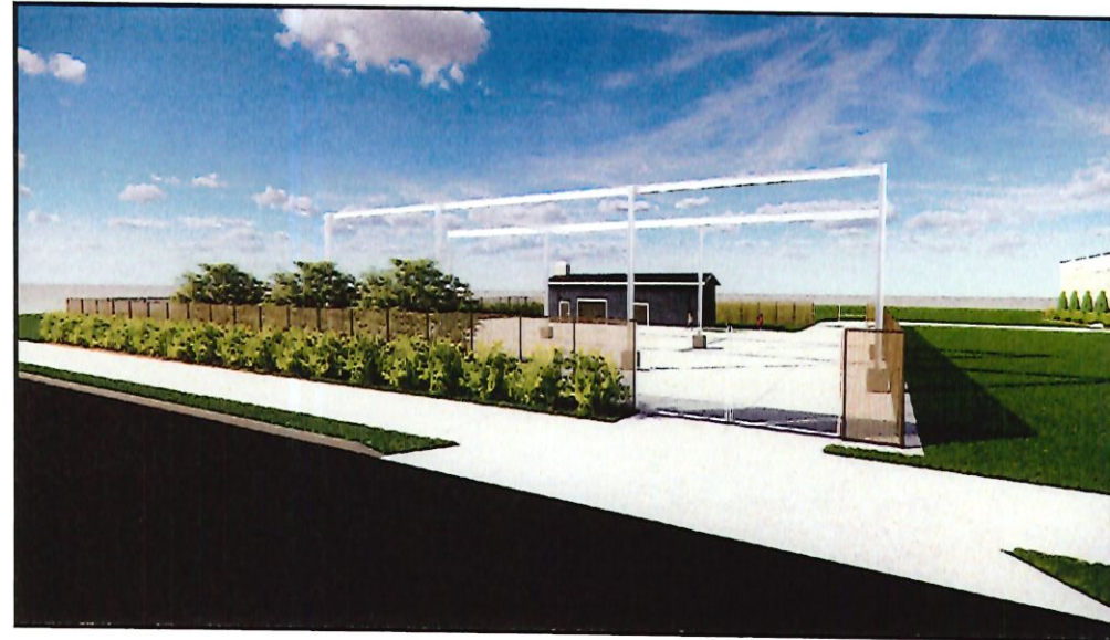
View 2 - Lift Station Site Rendering with Monorail System, Equipment Building, and Site Fence
